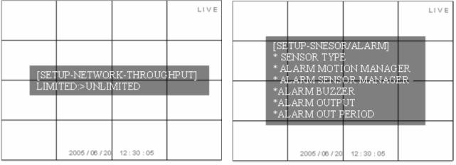
"NC" means normal close. If "NC" is chosen, the DVR will set off the alarm if the alarm is at high level.
